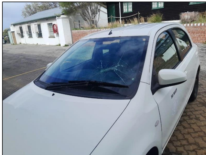
Figure 2. Damage to a car windscreen caused by a baboon jumping onto it from a height.
